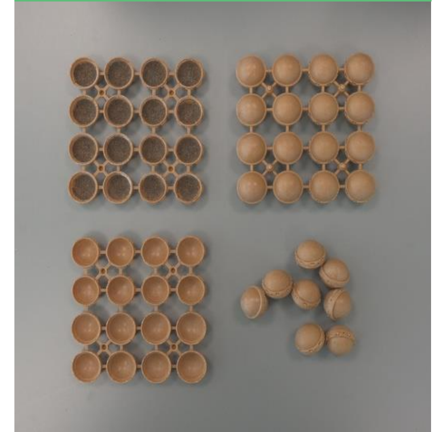
Production steps of OptiKugel
